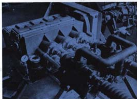
Steam-powered engine, before installation in bus. The three double-acting compound pistons at right have one high pressure and two low pressure cylinders.
