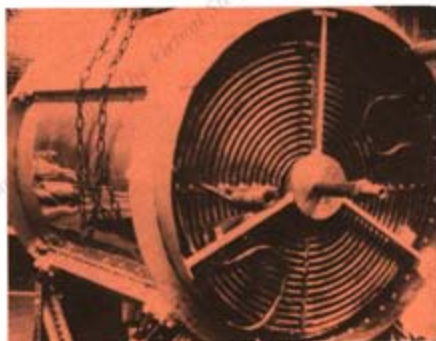
Steam generator, with flue end removed, shows monotube construction. A forced circulation of small amount of water and steam is induced through 1,400 feet of coiled steel tubing.
