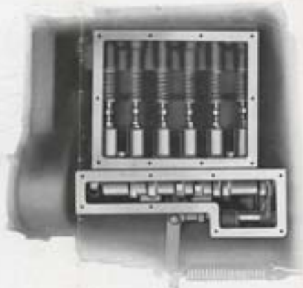
Engine Assembly, showing valves, cam action and accessibility
