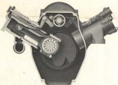
End View of V Engine, Showing Connecting Rod, Piston and Valve Action
