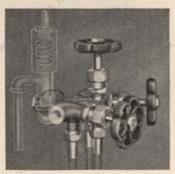
This improved blow off valve will clean pilot vaporizer and main vaporizer. The third valve is used for the syphon. To this valve is also attached the safety valve, and one plug. The plug may be used to attach a live steam coil entering the pump box to keep it from freezing in winter. The plug may also be used for a steam whistle.
