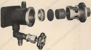
Can be taken apart for cleaning without removing from car and without releasing pressure from pressure tank. Replaces old style filter without change in tubing. Just drill two holes and connect. Pilot tank wrench opens from strainer. Lower valve shuts off filter from pressure tank.
