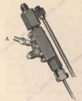
The Cruban Throttle is of a new and improved design throughout. Notice particularly the automatic by-pass or cylinder relief. When the throttle is closed, the pressure in the steam chest and cylinder is immediately by-passed to the condenser through connection A. This means a great saving in effort and brake lining, and considerably added safety, particularly when backing in close quarters.
