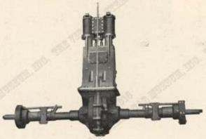
The engine is of our own construction, of the double cylinder, double acting type, and is directly connected to the rear axle by a spur gear, being geared three to one. The rear axle gear case and aluminum engine frame unite forming an oil tight and dust proof chamber in which are enclosed all of the moving parts, which are lubricated on the splash system. Ball bearings of a large size are used in the crank shaft and crank pin bearings.
