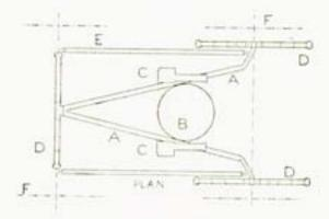
Reaches, E, hold front and rear axles parallel. Wheels, F, of wood, 30 in. diameters. Special metal hubs, 1\frac{1}{4} in. rear and 1\frac{1}{8} in. front, have a 52 in. track, 60 in. wheel base. Rocker pivot, G, under front spring D, provides for uneven ground without wrenching.
