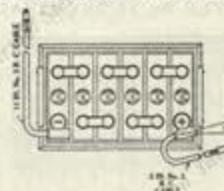
Add  $\frac{1}{8}$  inch to length to determine length over handles; if handles are on side of box add  $\frac{1}{4}$  inch to width to determine width over handles.
