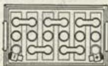
Add  $\frac{1}{8}$  inch to length to determine length over handles; if handles are on side of box add  $\frac{1}{4}$  inch to width to determine width over handles.
